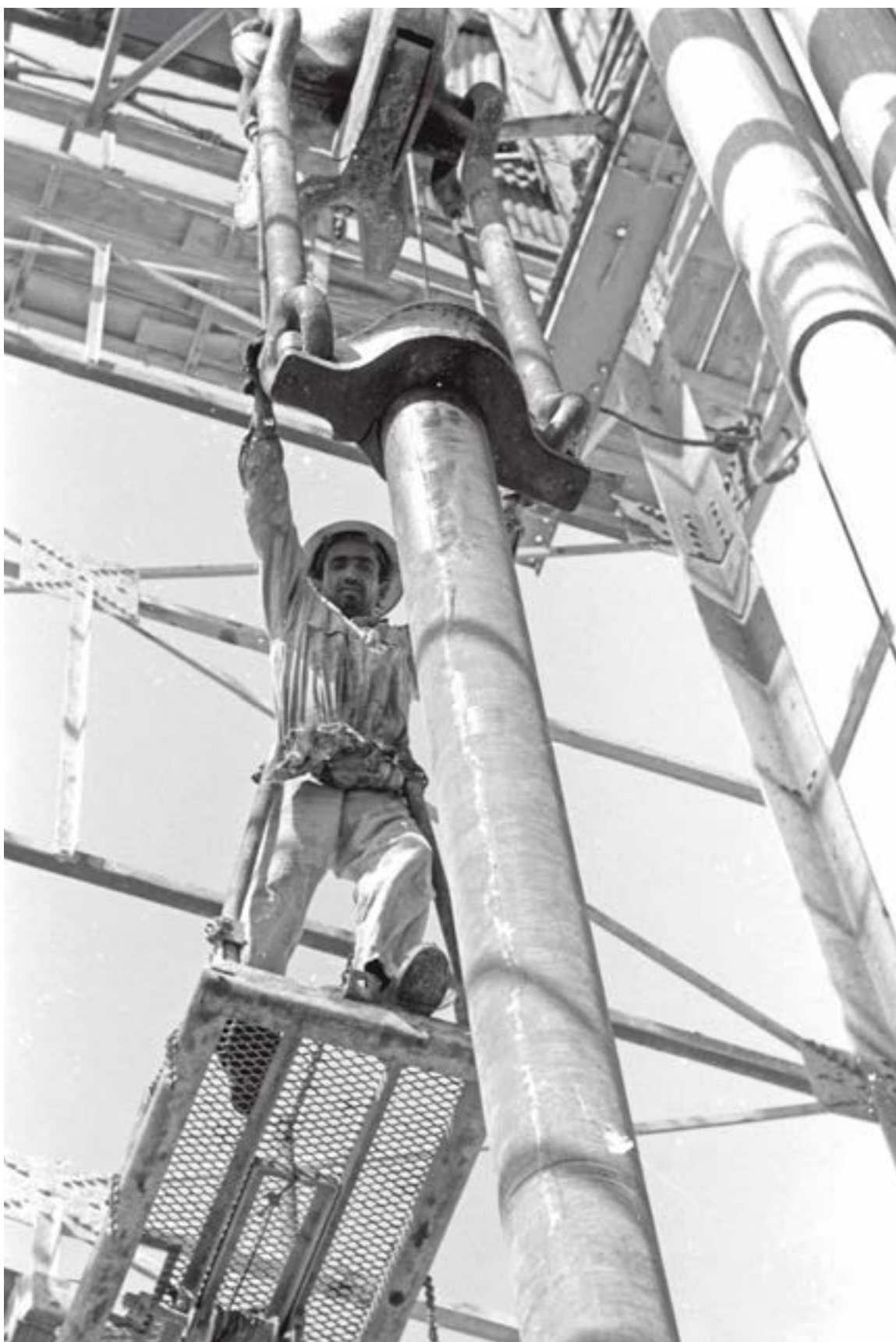
Guide cementing head at Manifa rig no. 11. Manifa, March, 1963. Photo by B. H. Moody
